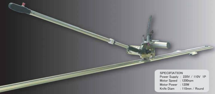
Cutting Head : Motorized Cutting Head
