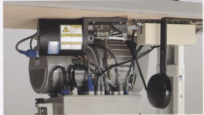
Automatic stitch fastening device TS2 Sews tying stitches (chaining-off stitches) at the sewing end to give a more stable finish with no unravelling. This device include automatic presser foot lowering device (including complete set of knee switch).
